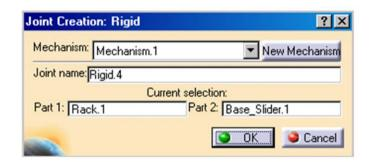
Similarly create a 'Rigid' joint between 'Base\_Slider.1' and 'surface\_To\_Be\_Checked.1'.
