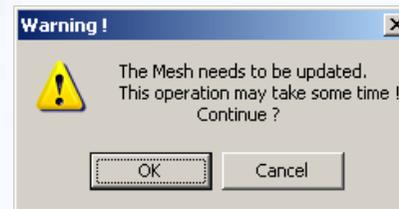
The minimum mesh size value 0.2 mm is a purely theoretical limit above which you are sure to be able to create a mesh. If you have less than this value, may or may not be able to create a mesh. This will be indeterminate because will depend upon the geometry.
