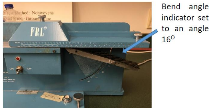
Figure 6. Pierce cantilever bending test device. Due to the stiffness of the woven carbon fabrics, the angle indicator is set to 16°.
