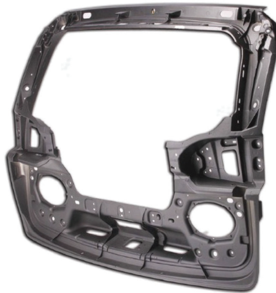
Figure 11.21: A magnesium liftgate for a 2017 Chrysler Pacifica, saving more than 10 kg in weight over the previous generation steel stamping, and with reduction of welds from 84 to 10. Magnesium is increasingly used for vehicle lightweighting, and high-pressure die castings such as this one can be produced with thin walls and intricate part details. Source: Courtesy of American Foundry Society.
