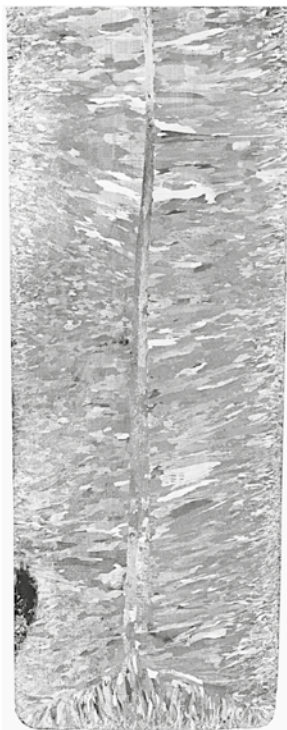
FIGURE 13.5 Internal structure of a cast metal bar showing the chill zone at the periphery, columnar grains growing toward the center, and a central shrinkage cavity. (Courtesy Ronald Kohser.)
