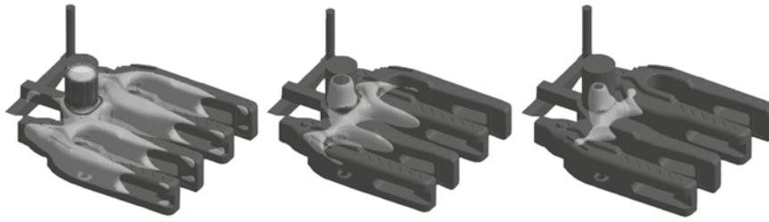
FIGURE 13.23 Computer model showing the progressive solidification of a cast steel mining shovel adapter. As time passes (left-to-right) the material directionally solidifies back toward the riser at the left side of the casting. Light material is liquid; dark material is solid. (Copyright 2009, Giesserei-Verlag GmbH, Dusseldorf, Germany.)
