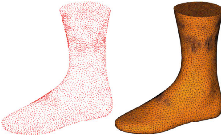
Fig. 1.10 Point cloud of a scanned surface (left) and a triangle mesh (right)
