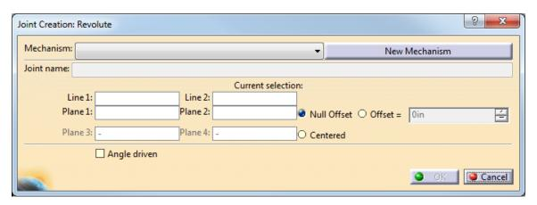
Mechanism Specifies the mechanism for the joint to belong to, you have the option of defining a New Mechanism
