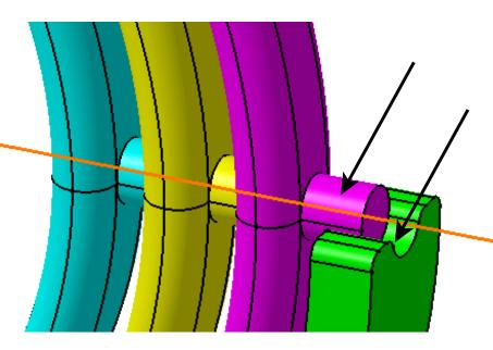
**Select the** zx plane in both parts. This defines the location of each object by aligning the two planes. You will probably have to expand the branches of the Base and  $I^{st}$  Ring in order to select the planes.
