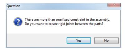
**Select** *Yes.* Two rigid joints were created and added to your mechanism. You should notice that the two components that are in the first pair are highlighted in the graphic area.
