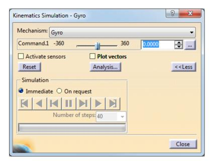
Turn on the *On request* option and drag the slider for *Command.1* to the right to 360. This will tell it to simulate one revolution.
