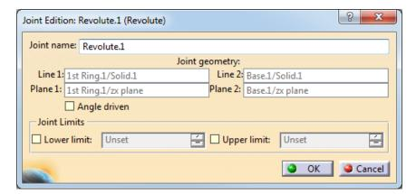
Joint Limits Sets limits for the range of motion if you turn on the Angle driven option
