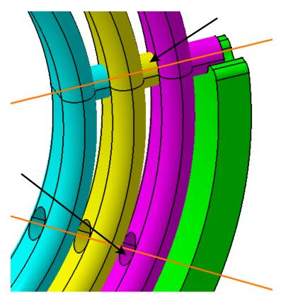
Select the zx plane in the  $2^{nd}$  Ring and Plane.1 from Geometrical Set.1 in the  $1^{st}$  Ring, turn on the Angle driven option and select OK. The middle ring moves to have the two lines line up. An Information window appears.
