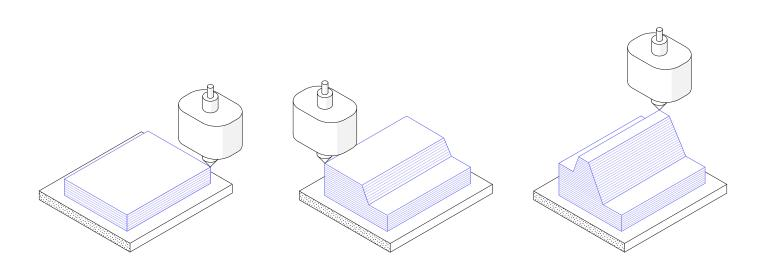
Every 3D printer builds parts based on the same main principle: a digital model is turned into a physical three-dimensional object by adding material a layer at a time.
