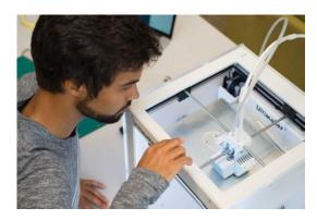
In FDM, a spool of filament is loaded into the printer and then fed to the extrusion head, which is equipped with a heated nozzle. Once the nozzle reaches the desired temperature, a motor drives the filament through it, melting it. The printer moves the extrusion head, laying down melted material at precise locations, where it cools and solidifies (like a very precise hot-glue gun).
