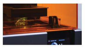
SLA and DLP are similar processes that both use a UV light source to cure (solidify) liquid resin in a vat layer-by-layer.
