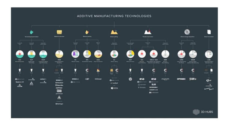
This infographic illustrates the seven 3D printing categories, the main materials each group can print with and the most popular printer manufacturers. The ISO/ASTM 52900 standard categorized all different types of 3D printing under one of these seven groups:
