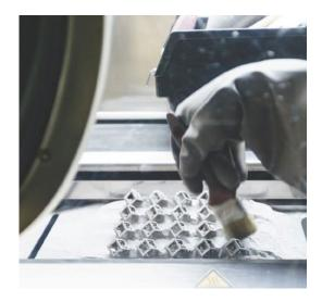
Direct Metal Laser Sintering (DMLS) and Selective Laser Melting (SLM) produce parts in a similar way to SLS: a laser source selectively bonds together powder particles layer-by-layer. The main difference, of course, is that DMLS and SLM produce parts out of metal.
