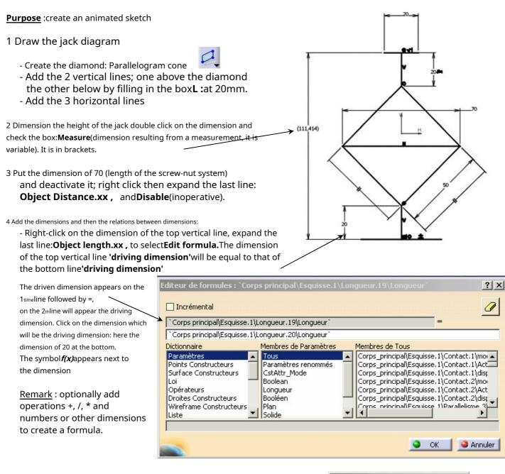
5 Complete the constraints by selecting the top horizontal line and the upper point of the top vertical line then add constraints and check:
