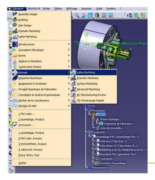
Open the ph20.CATProduct assembly file and launch the "Lathe Machining" workbench
