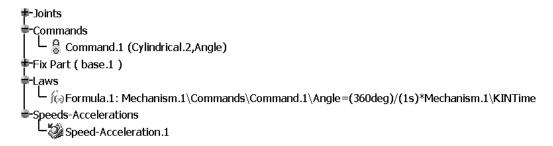
Having entered the required kinematic relation and designated the vertex on the block as the point to collect data on, we will simulate the mechanism. Click on **Simulation with**
