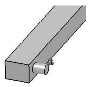
Next, we will create a coincident edge constraint between the base and the block. This removes all dof except for translation along the edge of coincidence and rotation about the edge of coincidence. The two remaining dof are consistent with our desire to create a cylindrical joint between the block and the base. To make the constraint, pick the
