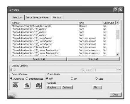
Observing that the coordinate direction of interest is X, click on the following items to record position, velocity, and acceleration of the block:
