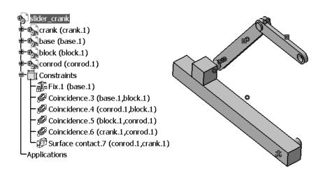
We need to apply one final constraint to locate the lower end of the crank onto the cylindrical protrusion on the base. Pick the **Coincidence** icon from **Constraints** toolbar. Select the axis of the cylindrical surface and the hole as shown below.
