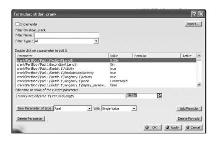
Point the cursor to the **Mechanism.1, DOF=0** branch in the tree and click. The consequence is that only parameters associated with the mechanism are displayed in the **Formulas** box.
