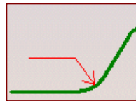
Limit Angle: Minimum angle between two segments that needs cornerization on the Side finish pass
