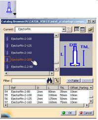
• Pick one of the points of the sketch previously created. You can see that the system has positioned an Ejector Pin on each point of the Sketch.
