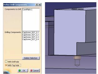
• Put the *CapScrews* in Noshow. Define some transparency in the graphic properties of the *Retainers*. You can now better check the drillings in the *Retainers* and *CorePlate*.
