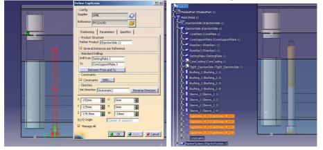
• Hide one of the screws. You can see that *SettingPlate* and *Risers* have been drilled with standard holes, while the last plate (*CoreSupportPlate*) has been bored with a threaded hole.
