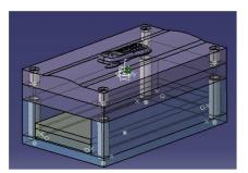
Double-click part *EjectorPlateA* in the tree. Make sure that *Geometrical Set.2* is the current active body (*Define In Work Object*).
