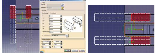
Switch to *Back View*. Make sure that no object is selected (no orange highlight). Make sure also that you will not pick the positioning grid. Then click the Slider in the 3D viewer : some of the dimensions of the Retainers are automatically adjusted to fit the Slider.
