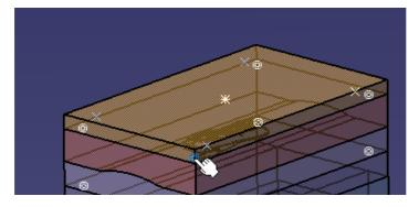
• You can see that the system has automatically recognized all four predefined points intended for positioning the Leader Pins. All instances are highlighted in red, which means that all of them are active : each further positioning operation will therefore apply to all of them simultaneously.
