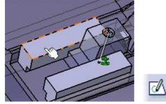
Create four points to be used as locations for the screws. Define constraints to the sides of the Retainers (choose the value).
