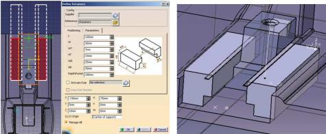
You can see that the height of the *Retainers* is not adequate because some material if left above them. Edit *Retainers* Component and set parameter HR = 35 mm for example. Validate modification and check result.
