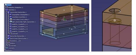
• Note also the automatic creation of Technological Results in the *ClampingPlate* and *CavityPlate*, conveying the technological information of the *DrillHoles* of the *LeaderPins* impacting the plate.
