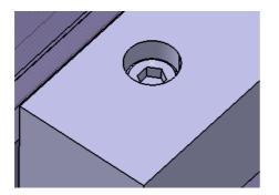
• Similarly, use again *the same function* to drill the *CorePlate* with the *TapHole* of all the *CapScrews*
