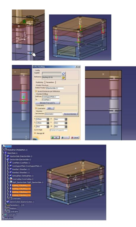
1.5 - Proceed similarly to create the appropriate Sleeves for these Leader Pins. Select reference Sleeve-32-120. Drill from SettingPlate to CoreSupportPlate and adjust W value to 15 mm (note that W position is adjusted in a single operation for all Sleeve instances, thanks to option Manage All).
