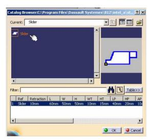
Click the top planar face of the Core Plate located in front of the rectangular hole in the area where the Slider mechanism is required.
