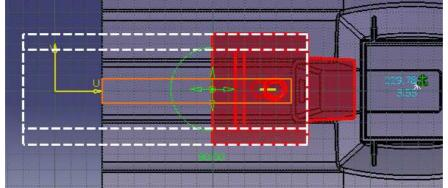
Display tab *Parameters* in dialog box *Define Slider*. Check the meaning of the following parameters in the panel picture and set them to the values mentioned : W=30mm, WT=7mm, HT=10mm, WF=25mm
