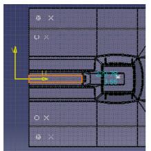
The system has switched to the sketcher-like view for positioning the component. Pick a point anywhere on the previous face : a preview of the Slider is displayed.
