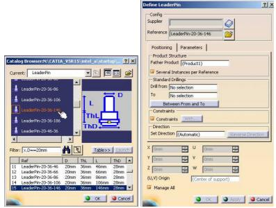
• Pick one of the predefined points located in the corner of the ClampingPlate in order to position the first instance of the Leader Pin :
