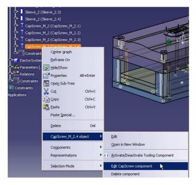
• Select tab *Parameters* in dialog box *Edit CapScrew*, activate design table icon corresponding to parameter L (length) and select reference *M12\*150*
