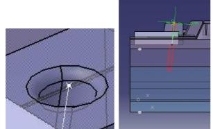
Drill *From CavityPlate To CorePlate*. The W position will be adjusted later via Edit capability. Validate creation.
