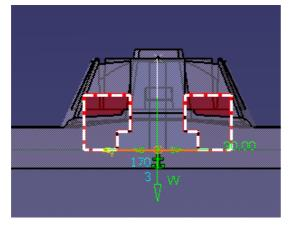
Switch to *Top View*. Define plates Drill from *CorePlate* To *CavityPlate*. Adjust the position and the length of the Retainers to ensure adequate contact length between the Slider and the Retainers. Define for example : L=100mm, X=-190mm, Y=5mm, Z=10mm. Validate creation.
