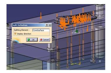
• Validate and zoom onto Ejector Pins area to check the result. Note that Split operation has automatically adjusted the fitting length of each Ejector Pin to take into account the value defined in parameter *Offset\_Parting*. You can measure it with function *Measure Between* : fitting length is computed using intersection of the center of the Ejector Pin with the Core Plate, but you can select the top edge of the drilling in the Core Plate in order to get an approximate result.
