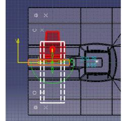
Adjust the position of the Slider by rotating it using the green half-circle.
