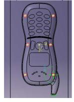
• Note that option *Several Instances per Reference* is not active (the value shown is the one defined in the Settings). This will ensure that each *EjectorPin* is created as a reference and can therefore be handled individually for splitting purposes later on.
