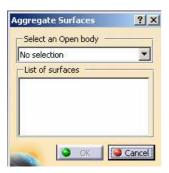
• Select Geometrical Set *Core* in the specification tree or pick anywhere in the red area in the 3D viewer.
