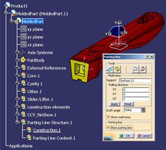
• Click the Reflect line icon in the Parting line dialog box and create the Reflect line.
