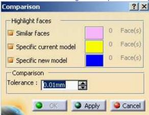
• The faces of the first and of the second Part are compared and classified into 3 groups: identical faces, faces specific to version no.1, faces specific to version no.2.
