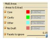
Now we have to transfer the remaining surfaces into the relevant areas. First, activate the *Lock* option.
