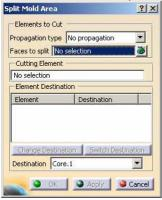
• Select *Propagation type : Tangent continuity.* Pick one of the faces impacted by the splitting curve as *Element to cut.* Pick the previous *Reflect line.1* as *Cutting Element.* Click *Apply.*
