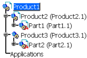
Figure 11-37 The Specification Tree having a product and a component within an assembly file.
