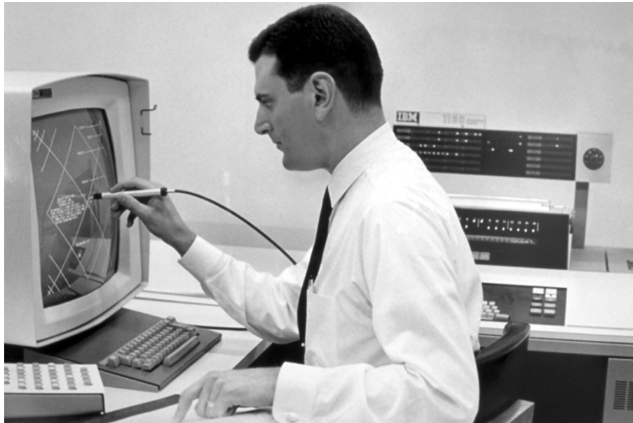
Figure 13.5 IBM 2250 Display Connected to an IBM 1130 Computer 8
