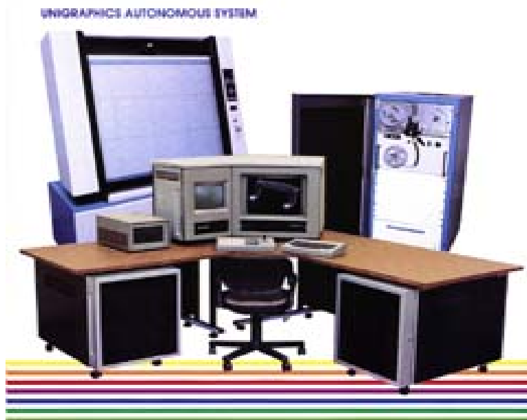
Figure 19.5 Low-Cost ADS-100 System (plotter and paper tape reader/punch were optional)
